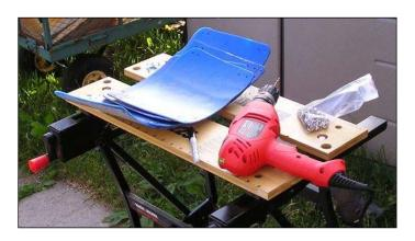
Finally, take the utility knife and de-burr the drill holes. Any plastic burrs will get in the way of the rivets.
